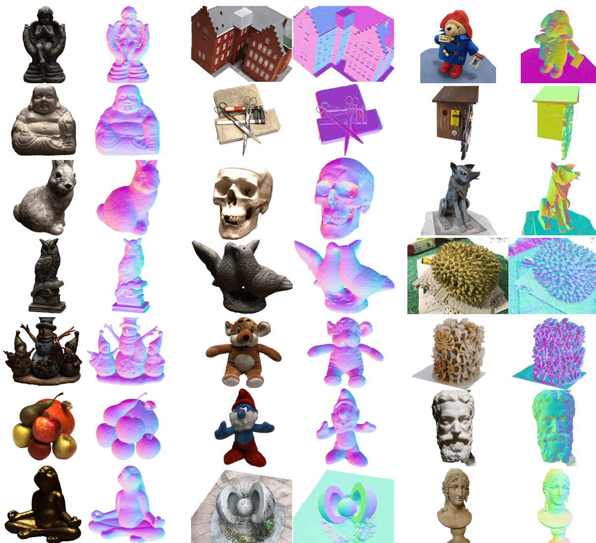
Fig. 12. Reconstruction showcase. Surface rendering and normals of various scenes from the DTU and BlendedMVS datasets, reconstructed with our algorithm and a decaying Laplacian. All results were generated with the same hyperparameters and a training time of \sim 1 minute per scene.
