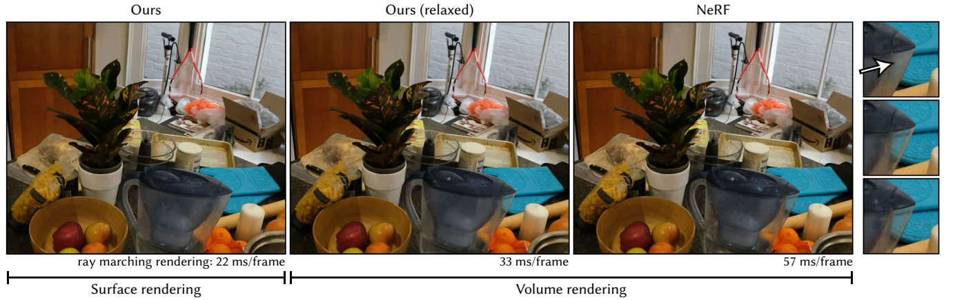
Fig. 10. Volumetric relaxation. We compare reconstructions of our method without and with volume relaxation to NeRF, all implemented in Instant NGP using the same hyperparameters. While our method achieves comparable visual quality using a surface-based representation, we highlight a region (white arrow) where it fails to model a semi-transparent object due to the opaque surface assumption. The relaxed variant of our algorithm can recover by adopting volume rendering in such regions. Rendering the reconstructions using the same ray marching implementation leads to significant performance differences: our surface-only reconstruction is 2.6× faster than NeRF. The relaxed variant benefits from the surface representation in most regions, and is 1.7× faster.
