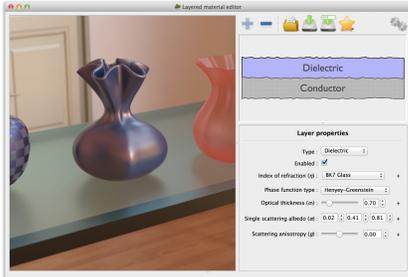
**Figure 12:** We developed an interactive visual design tool to explore the space of layered BRDF models; the supplementary video shows an editing session using it.
