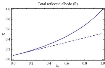
**Figure 11:** Comparing the total reflected energy  $R$  of a smooth dielectric  $\eta = 1.5$  on top of a Lambertian surface with reflectance  $k_d$ . A recent approximate model (dashed) proposes a linear relation between  $k_d$  and total reflectance, which is not seen in the exact solution that considers all orders of interreflection.
