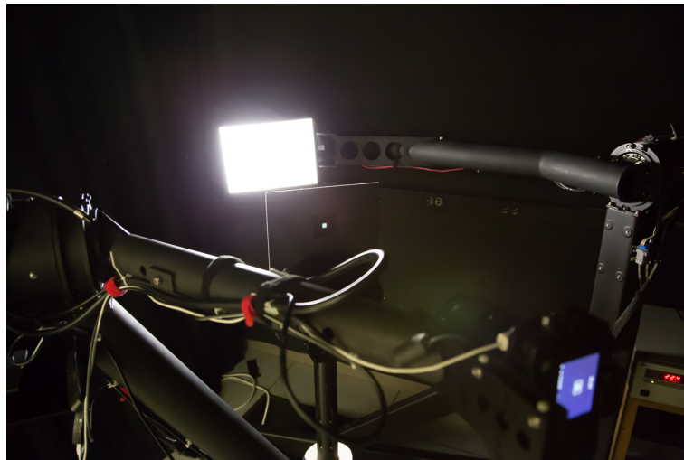
Figure 25: Photograph of our measurement setup: a small swatch of enamel mounted at the center of a spherical gantry is illuminated by a rotating rectangular light source, while the camera measures the radiance along the normal direction
