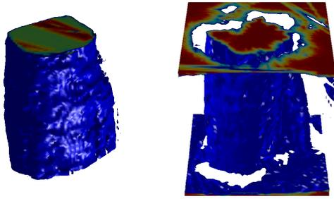
**Figure 9:** The visual hull obtained using the bluescreen (left) is useful as a rough bounding shape, but fails to capture geometric depressions. The space carving volume is more accurate in this regard, but suffers from many areas incorrectly labeled as occupied. We combine the two volumes to remove both of these problems.
