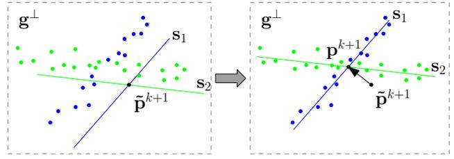
**Figure 8:** A correction step adjusts the position in the plane perpendicular to the current growing direction. The offset is chosen to align hair observations with a model predicting their positions along a set of lines corresponding to the different camera angles.
