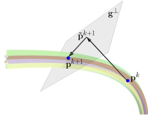
**Figure 6:** Our algorithm iteratively moves along a hair identified by the common intersection of a set of mutually intersecting ribbons. This is done by repeatedly estimating the local fiber direction and taking a step, after which a correction moves the position back onto the centerline.
