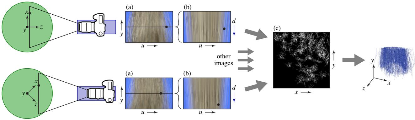
**Figure 2:** Our capture proceeds by taking several sets of photographs, each consisting of a sweep of the camera along the translation stage. (a) Example images from two sweeps, seeing the same hair rotated to a different angle. (b) Images plotting  $u$  against camera position reveal the 3D locations of hairs. (c) Features located from many sweeps are combined, forming stars that reveal the positions of the fibers.
