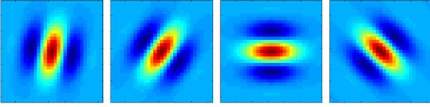
**Figure 5:** To detect the image-space orientation of in-focus hairs, each photograph is convolved with a large filter bank of rotated Gabor filters. The angle of maximum response serves as a estimate of the projected fiber direction.
