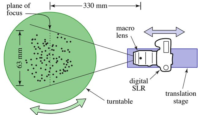
**Figure 1:** Our measurement setup consists of a digital still camera imaging a sample of hair through a macro lens. The hair rotates around a vertical axis, and the camera translates along its optical axis, which is perpendicular to the rotation axis.
