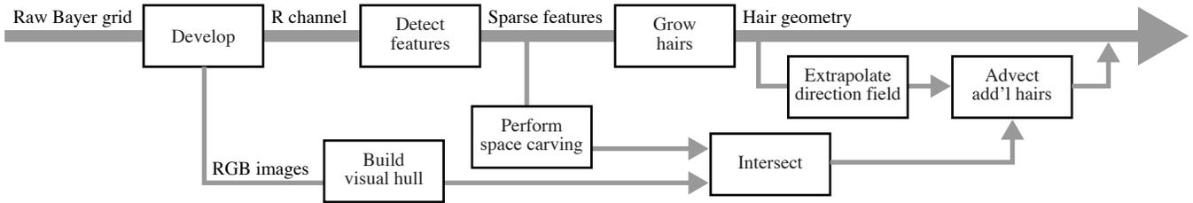
**Figure 4: Overview:** A ridge detection stage identifies well-focused hairs in each of the input photographs, after which three-dimensional fibers are grown through the resulting feature data. To fill in empty areas, occluded regions are identified using a space carving approach and additional fibers are then advected through an extrapolated velocity field.
